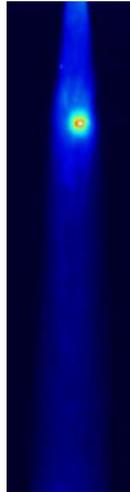
The suspension jet is absolutely concentrated and powerful in cutting. (Image: ANT AG. Thermal image: Leibniz University Hannover)
